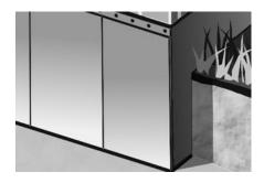
The top end of the waterproofing membrane is to be fixed at the basement level by profiled metal edge strip and sealed.
