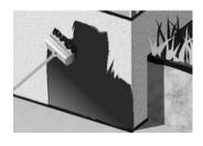
The surface must be smooth, dry, clean and with no oil stains. For better adhesion, treat the surface with primer.
